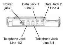
Line Jacks: Jack L1/L2 is used for telephone lines 1 and 2. Jack L3/L4 is used for telephone lines 3 and 4. Data jacks 1 and 2 are used to connect a fax, modem or other device through the NSQ412 to the telephone line.
